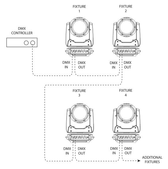
Note: The diagram above depicts DMX linking via the 3-pin DMX ports, but the units can also be linked via the 5-pin DMX ports. However, all linkages must be made using the same set of ports: all 3-pin or all 5-pin.
