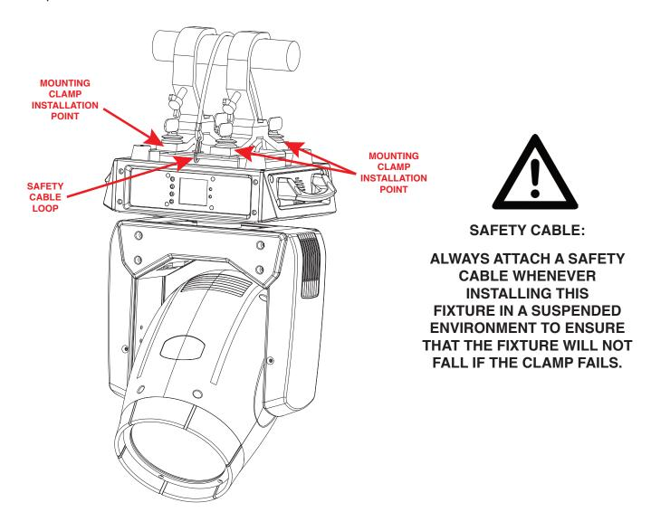
**NOTICE:** The maximum ambient operational temperature for this lighting fixture is *113° F (45° C)*. Do not place this lighting fixture in an environment where the temperatures exceed this value. This will allow the fixture to run at its best and help prolong the fixture life.
